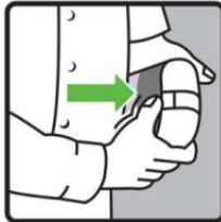
2. Remove unit by pulling yellow strap upwards.
